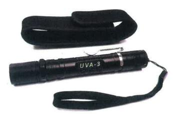
The **UVA-3** is a hand-held battery powered Ultraviolet inspection lamp used for a range of Non-Destructive Testing (NDT) applications. The filtered 365nm output makes it ideal for Fluorescent Magnetic Particle Inspection (MPI) & Fluorescent Dye Penetrant Inspection (DPI), as well as leak detection applications when used with a suitable additive (i.e. Spectroline Oil-Glo).
